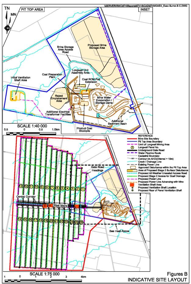
Once each set of dual roadways is fully developed, the longwall equipment would be installed and the coal recovered as the longwall unit retreats back towards the West Mains between the two sets of roadways. All coal would be conveyed back to the Pit Bottom Area for transfer to the surface via the approved conveyor drift.
